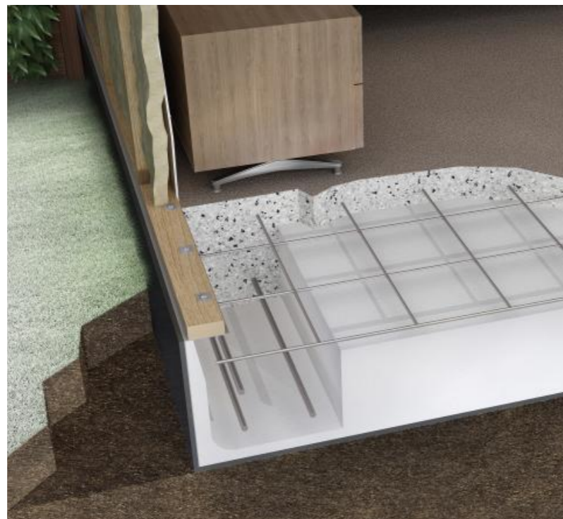
Fully insulated slab and foundation
